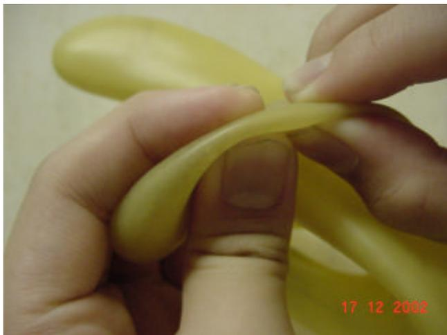
Figure 7 Pinching is to squeeze the gloves by fingers to pinpoint the irregularities of a small area.
