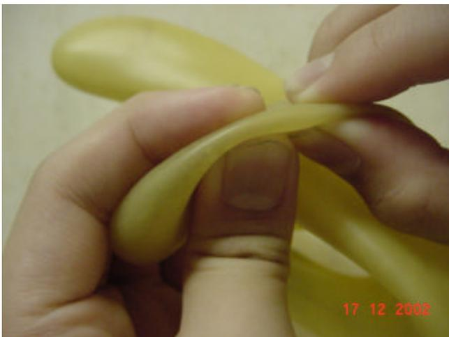
Illustration 5 Pinching is to squeeze the gloves by fingers to pinpoint the irregularities of a small area.
