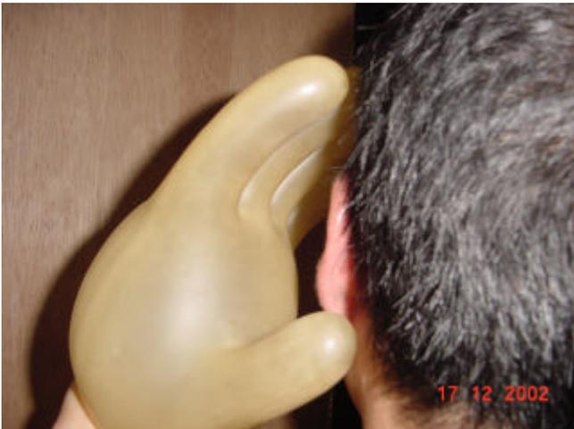
Illustration 3 Held the inflated glove close to the ear to detect for leaks
