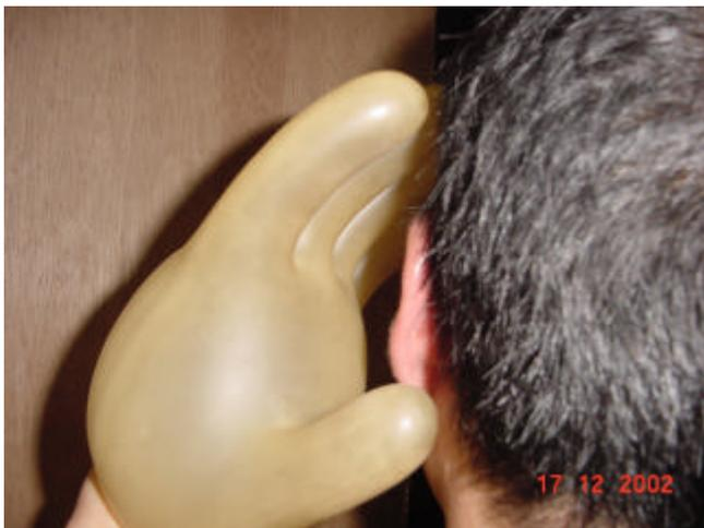
Figure 5 Held the inflated glove close to the ear to detect for leaks
