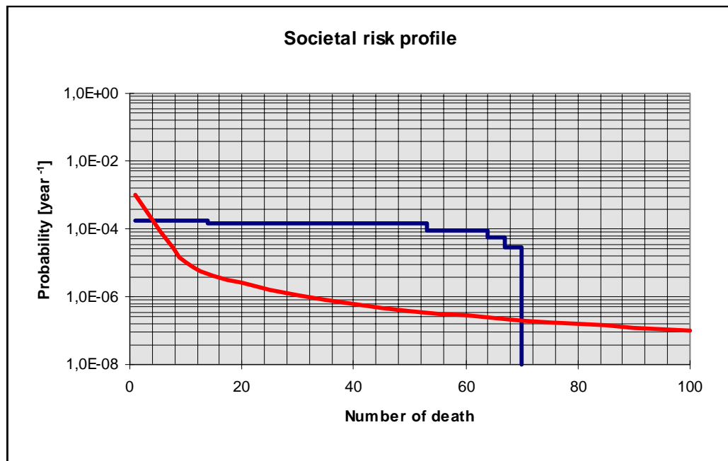
Figure 4.1: Comparison between Dutch acceptable risk level (red) and calculated societal risk level (blue).
