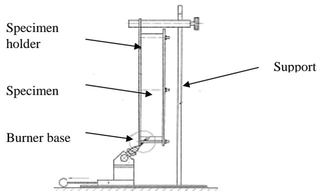
Figure 3.5 Setup for the Ignitability test apparatus
