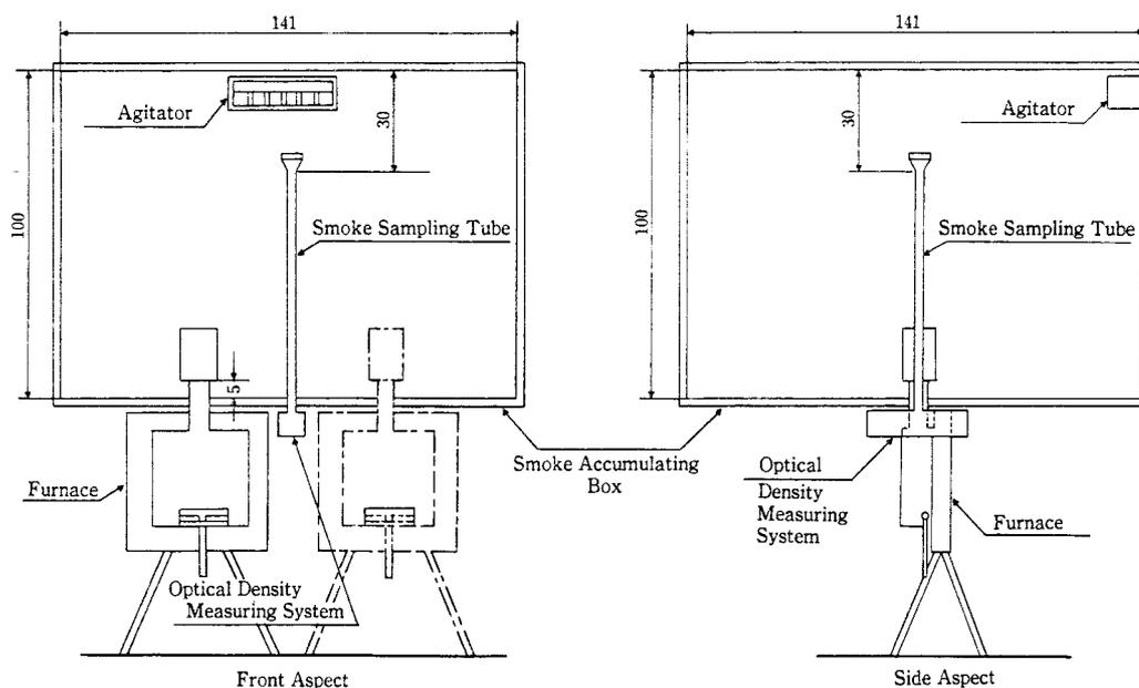
Figure 5.2 Typical set up of the Surface test /26/
