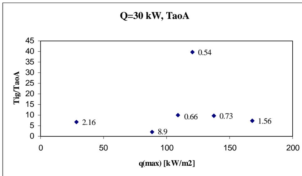
Figure B2  $T_{ig}/\tau_A$  plotted against  $q_{max}$  when the radiant heat flux is 30 kW/m<sup>2</sup>
