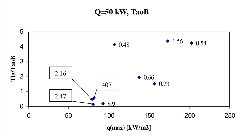
Figure B2  $T_{ig}/\tau_B$  plotted against  $q_{max}$  when the radiant heat flux is 50 kW/m<sup>2</sup>
