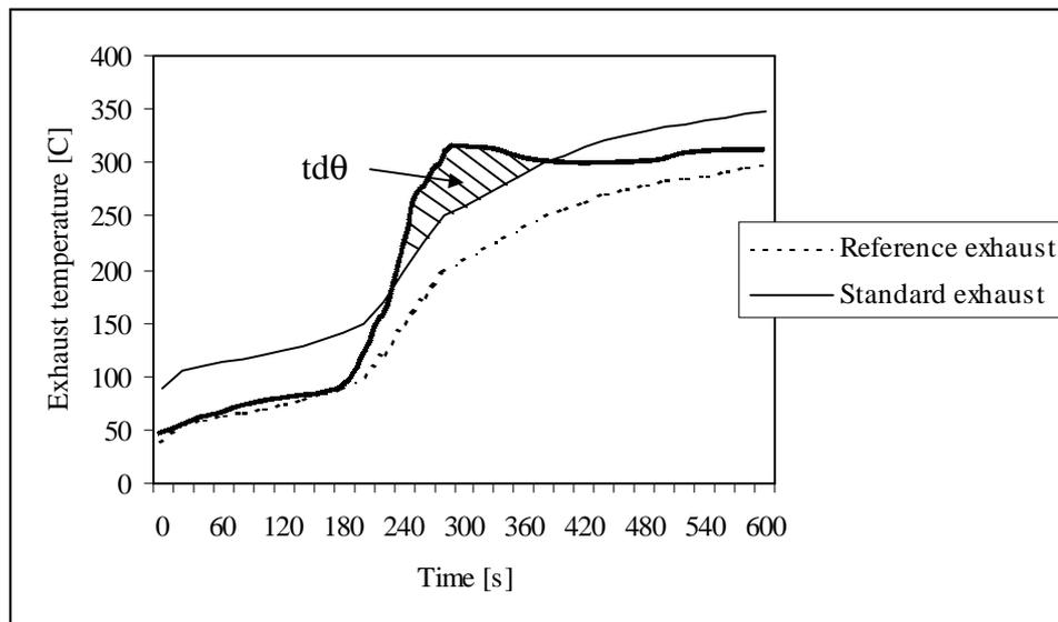
Figure 5.3 Definition of the  $td\theta$  value, the thickest line represents the tested material
