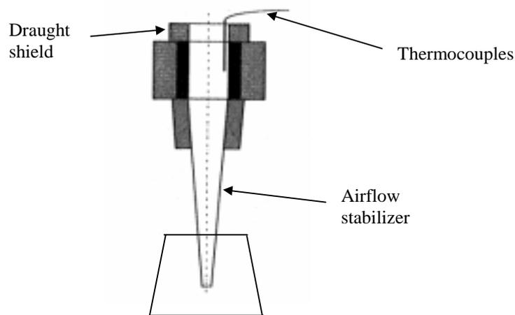
Figure 3.3 General arrangement of the Non-combustibility test /14/
