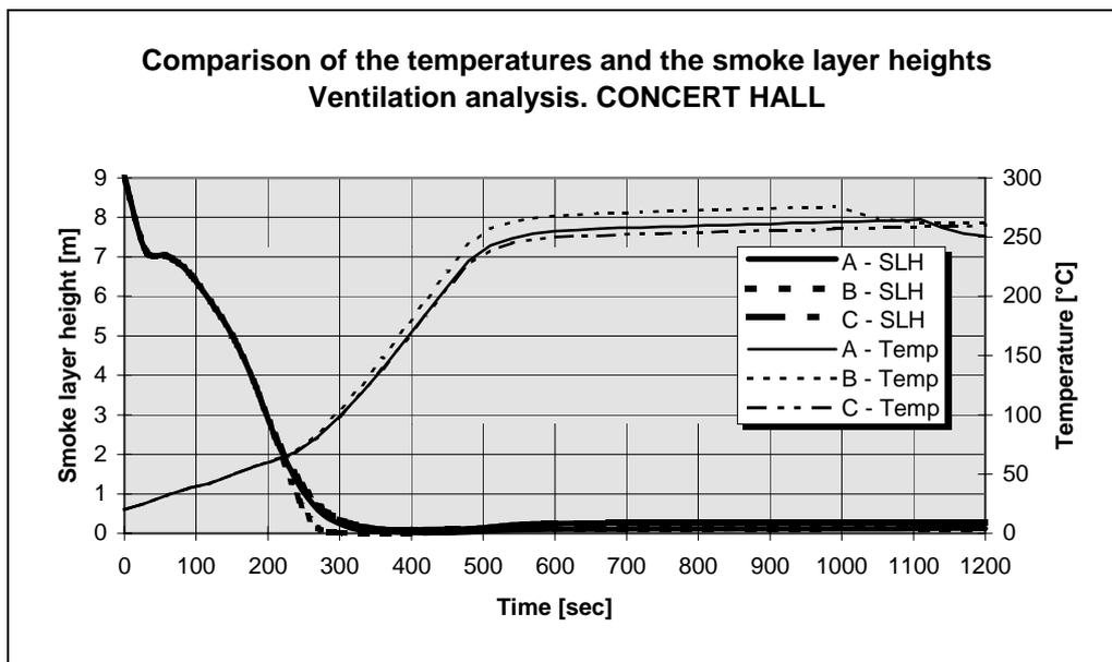
Figure 5.13: Comparison of the temperatures and smoke layer heights in Box 7 (Concert hall). Fictive fire in the concert hall. (A = all doors open, B = all doors to the outside and the foyer closed, C = three doors to the alley closed).
