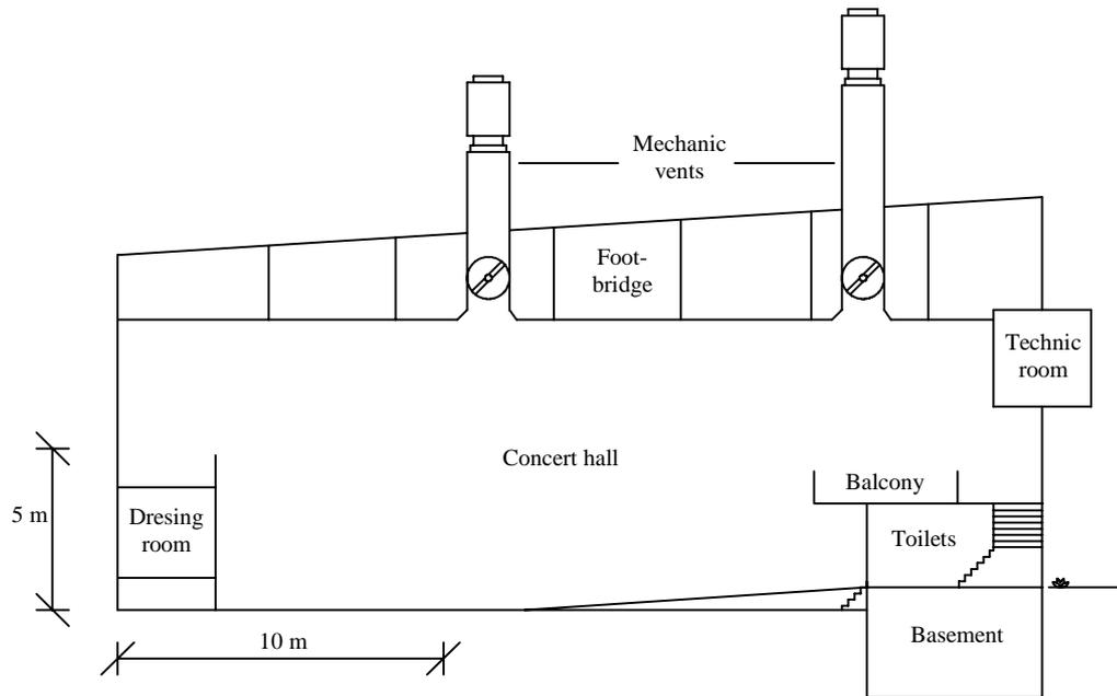
Figure 2.6: Sectional view of "Amager Bio".
