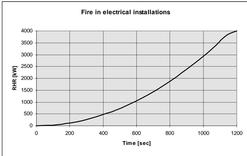
Figure 4.3: RHR for fire in the electrical installations.
