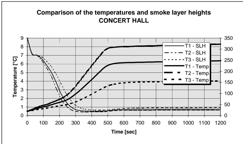
Figure 5.12: Comparison of the temperatures (Temp) and the smoke layer heights (SLH) in Box 7. (T1 = RHR, T2 = RHR+50%, T3 = RHR-50%).
