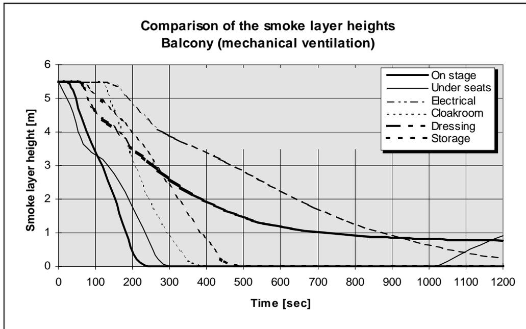
Figure 5.20: Comparison of the smoke layer heights on the balcony. Mechanical smoke ventilation activated. Results mapped for the different fire scenarios.
