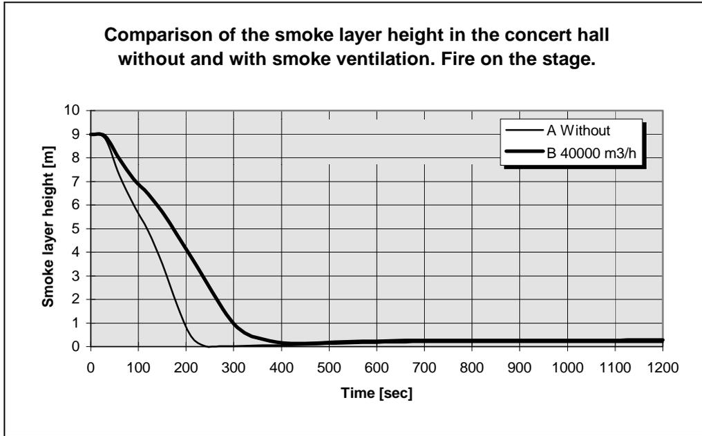
Figure 5.22: Comparison of the smoke layer heights in the concert hall. (A = no smoke ventilation and B = the present smoke ventilation  $11.1 \text{ m}^3/\text{s}$ ).
