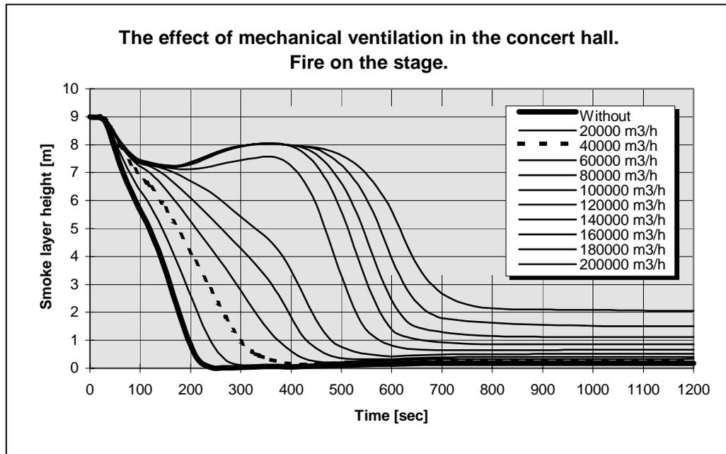
Figure 5.23: The effect of different mechanical ventilation flows in the concert hall. Fire on the stage.
