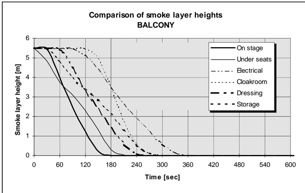
Figure 5.15: Comparison of the smoke layer height on the balcony.
