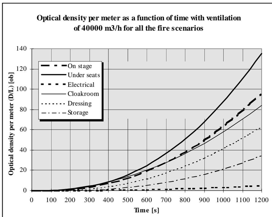
Figure 6.4: Optical density per meter as a function of time with ventilation of 40000 m<sup>3</sup>/h for all the fire scenarios.
