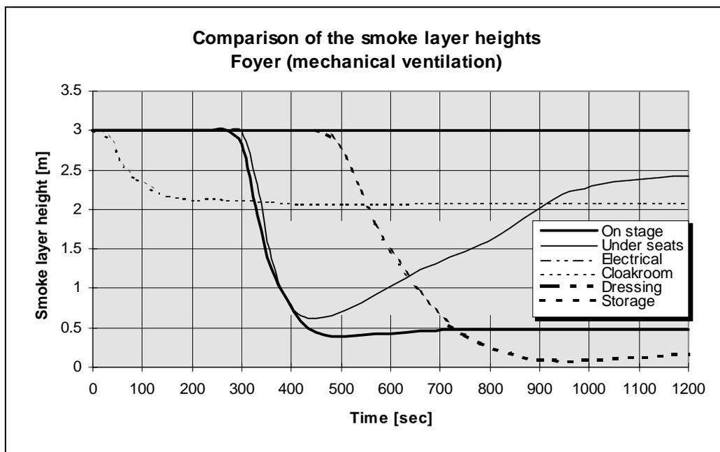
Figure 5.21: Comparison of the smoke layer heights in the foyer. Mechanical smoke ventilation activated. Results mapped for the different fire scenarios.
