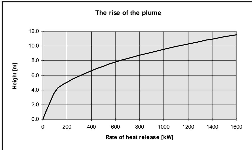
Figure 5.2: Rise of the plume as a function of the rate of heat release.
