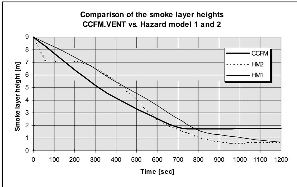
Figure 5.26: Comparison of the smoke layer heights in the concert hall with mechanical ventilation for the fire scenario “Fire on the stage” by usage of different models: CCFM.VENT, Hazard model 1 and Hazard model 2.
