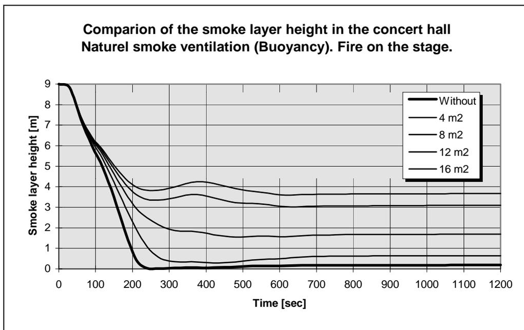
Figure 5.24: The effect of natural ventilation in the concert hall. Fire on the stage.
