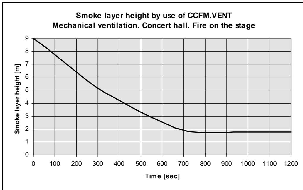
Figure 5.25: The smoke layer height determined by CCFM.VENT. Fire on the stage with mechanical ventilation of 40000 m<sup>3</sup>/h. Concert hall.
