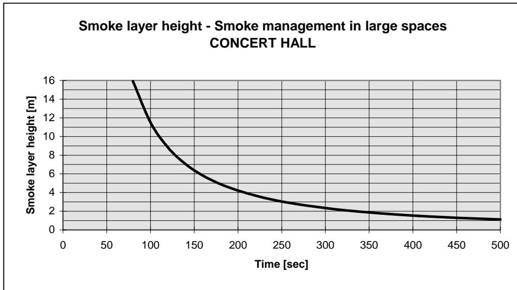
Figure 5.17: Fire on the stage. Smoke layer height calculated on experimental data.
