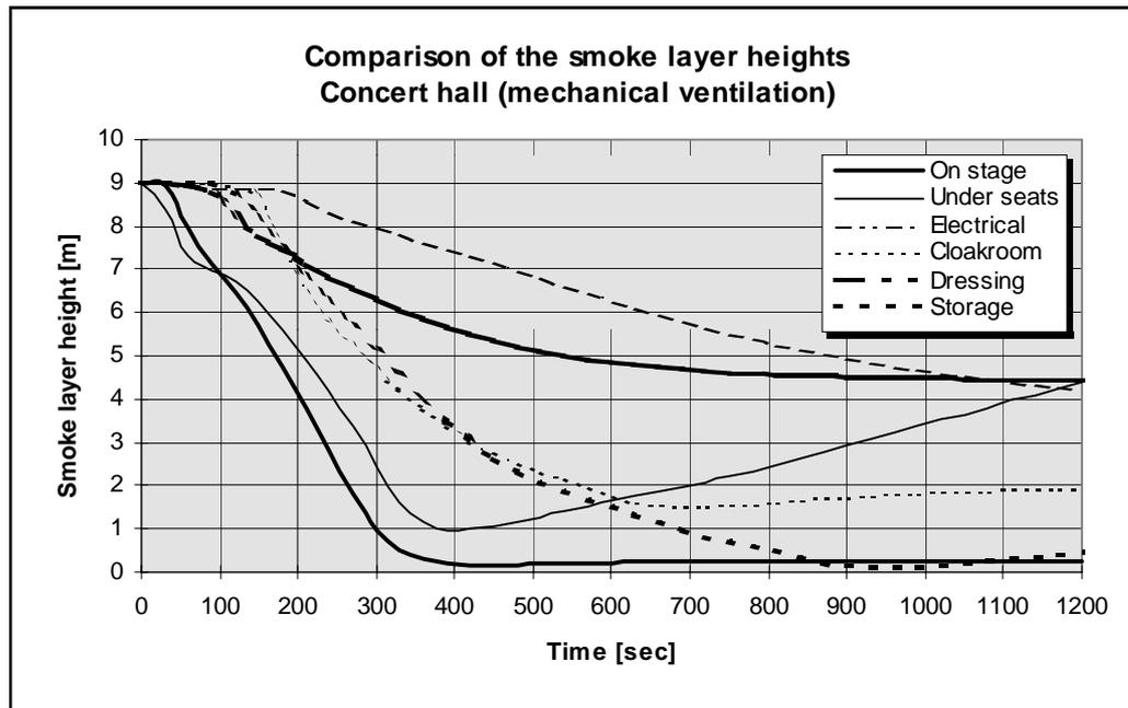
Figure 5.19: Comparison of the smoke layer heights in the concert hall. Mechanical smoke ventilation activated. Results mapped for the different fire scenarios.
