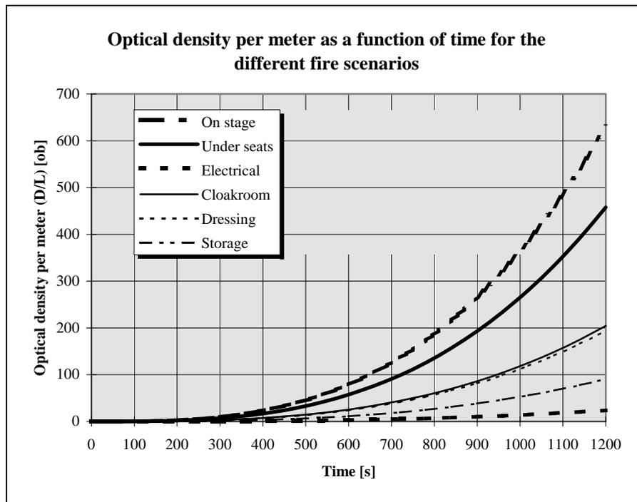
Figure 6.2: The optical density per meter as a function of time for all the fire scenarios.
