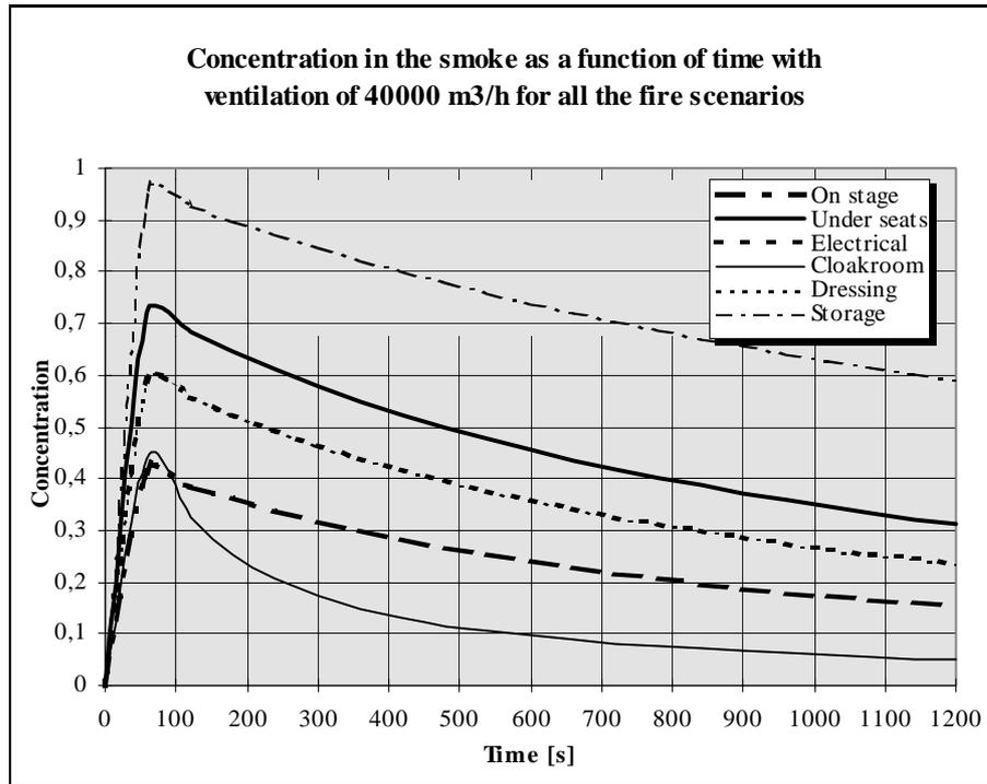
Figure 6.3: Concentration as a function of time with ventilation of 40000 m<sup>3</sup>/h for all the fire scenarios.
