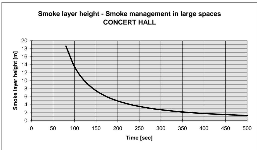
Figure 5.18: Fire under the seats. Smoke layer height calculated on experimental data
