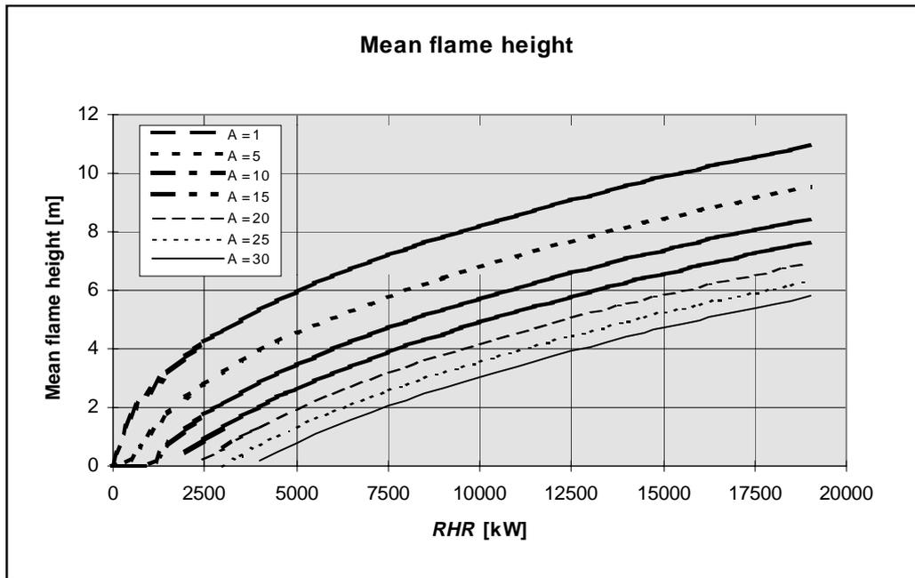
Figure 5.3: Mean flame height as a function of the RHR and the burning area.
