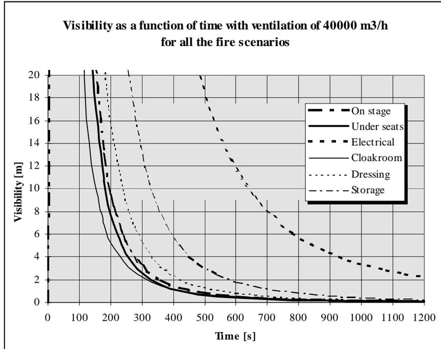
Figure 6.5: The visibility as a function of time with ventilation of 40000 m<sup>3</sup>/m for all the fire scenarios.
