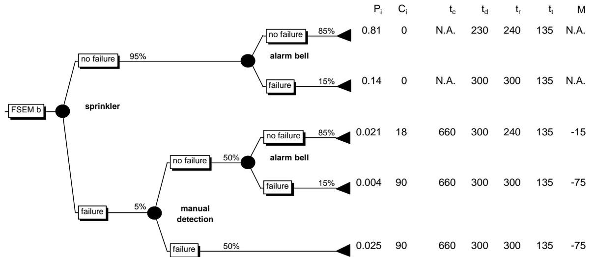
Figure A8 Event tree for Fire Safety Engineering Method B design.
